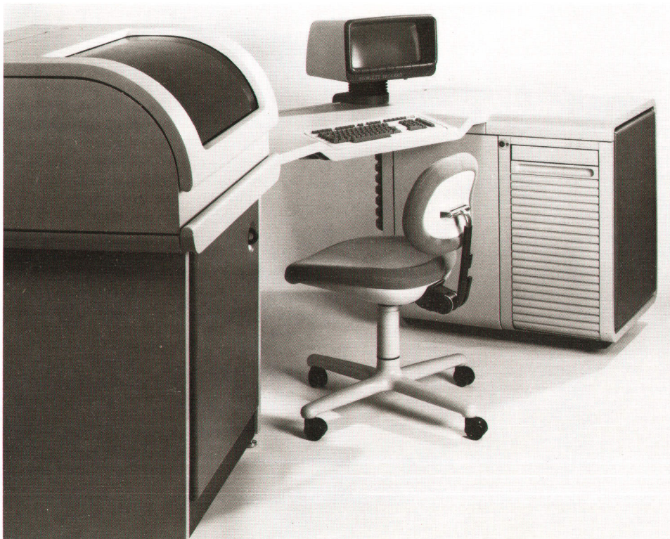
Fig. 1. The HP 250 is a low-cost entry level computer system for small businesses. It is shown here with the optional printer noise-reduction enclosure.
